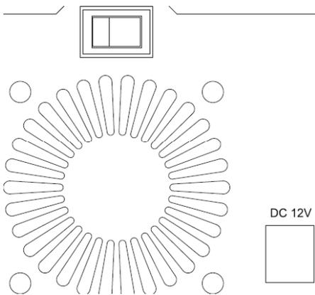
Adaptor is DC12V /5A input and Main Power can turn on/off DVR on Switch.
