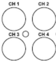
It connects video sources (camera image) to BNC connector via cable.
