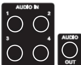
It connects audio source (mic) to audio input (4CH) of RCA and connects speaker to audio output.
