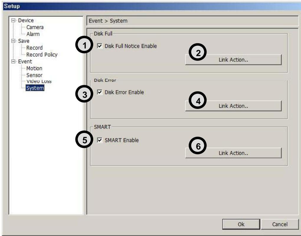
1 **DISK FULL** : List for all installed HDD disks.
